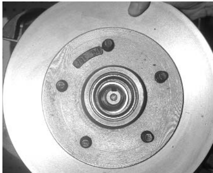
Mount the rotor with the installed inner bearing onto the rotor
