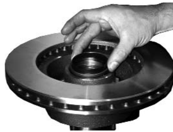
Install the grease seal into the rotor
