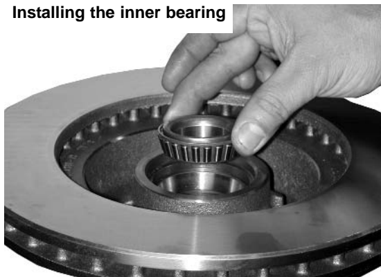
Installing the inner bearing
