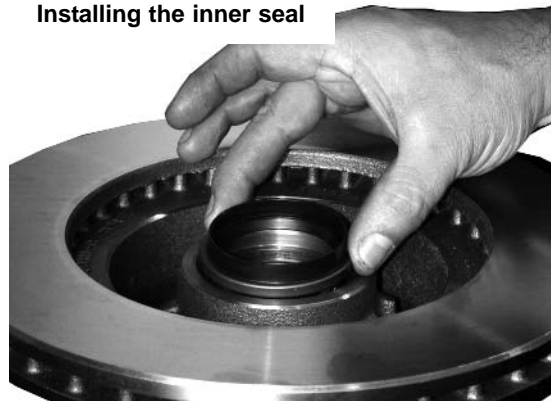
Installing the inner seal
