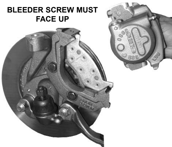
PASSENGER SIDE WITH CALIPER TOWARD REAR OF CAR. INSIDE VIEW.
