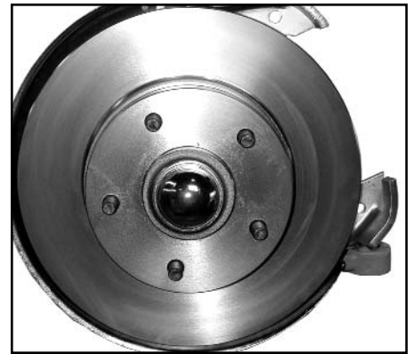
Install dust cap & clean rotor.
