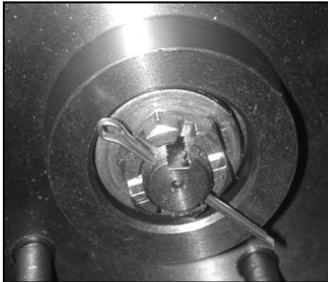
Install spindle washer, nut & cotter pin.
