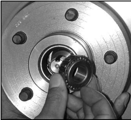
Install outer bearing.
