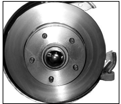
Install dust cap & clean rotor.
