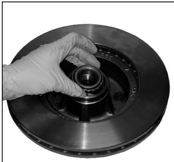
Install the inner A6 bearing.
