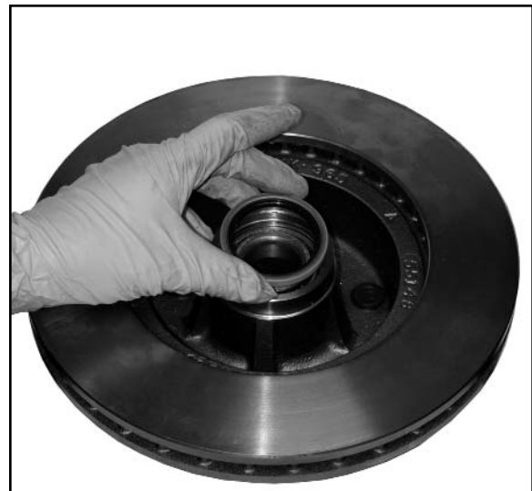
Install the bearing seal (HW7934).
