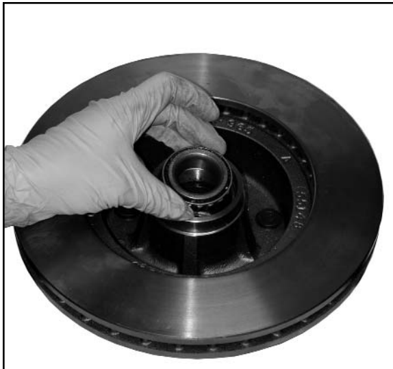
Install the inner A6 bearing.
