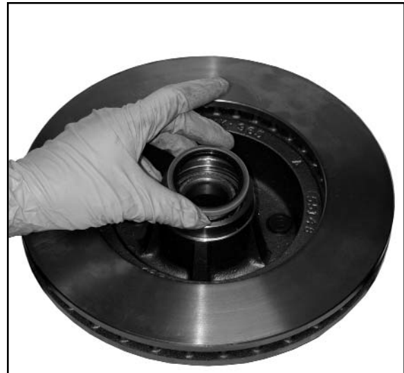
Install the bearing seal (HW7934).
