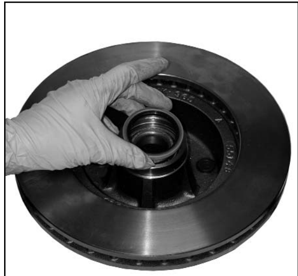
Install the bearing seal (HW7934).
