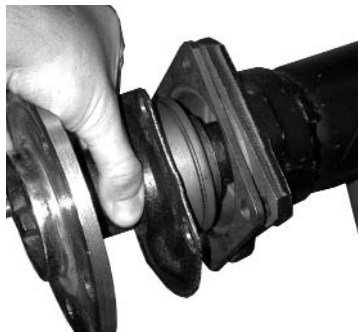
Remove axle flange retaining bolts - install axle into housing. Axle flange may need to be machined.
