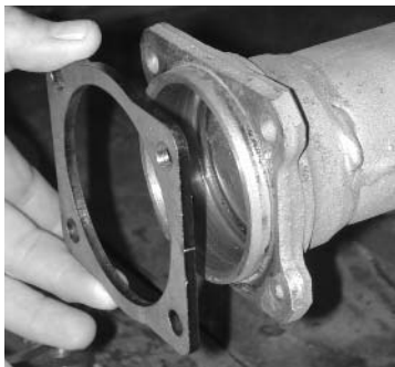
Install spacer plate to replace the backing plate.
