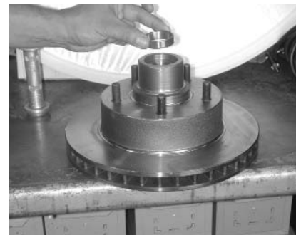
Install the new outer bearing race and tap it into the rotor securely
