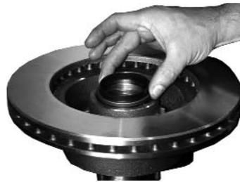
17. Grease the spindle where the bearings fit. Install the rotor onto the spindle followed by the outer bearing, the keyed washer and spindle nut. Tighten the spindle nut to the specified torque and insert the cotter pin. Bend the cotter pin, snip off the excess, and install the dust cap, by tapping a socket that fits on the cap edge, or by tapping a screwdriver on the edge of the cap. Spin the rotor and check to be sure that it rotates smoothly and there is no wobble. **Clean the rotor.**
