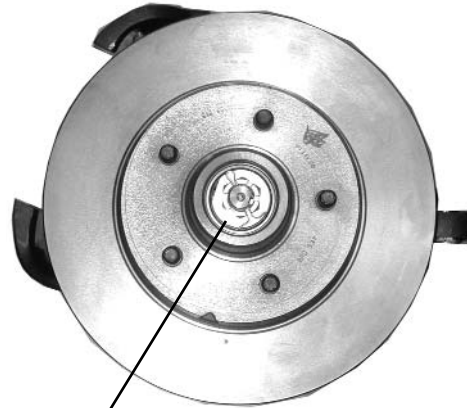
Notice the washer, nut, and cotter pin have been installed.
