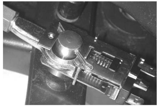
7. The brake pedal should be adjusted so there's about 1/4-1/2" free travel in the pedal before the booster rod moves.
