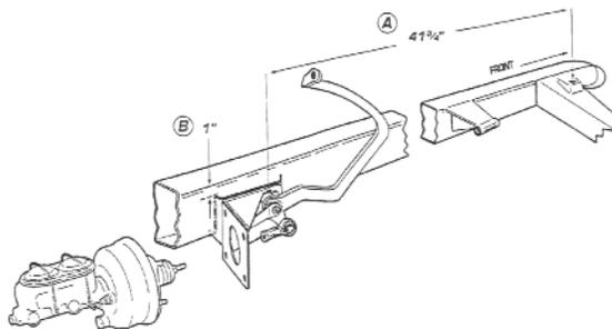
2. The top of the mounting bracket should be located parallel to and 1" below the top of the frame rail (B).
