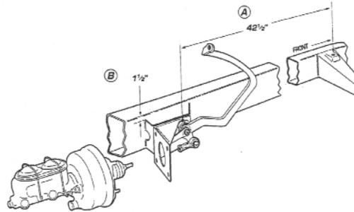
2. The top of the mounting bracket should be located parallel to and 1 1/2" below the top of the frame rail (B).
