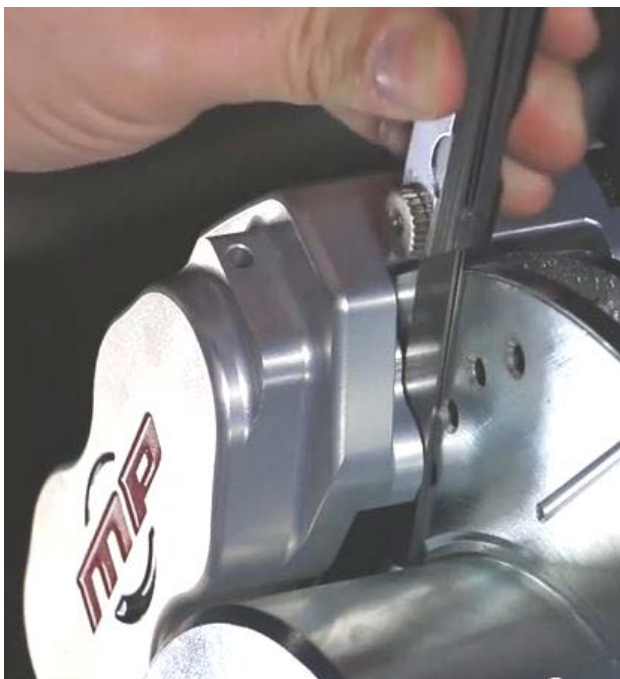
Figure 4a – Measuring the Caliper to Rotor Clearance
