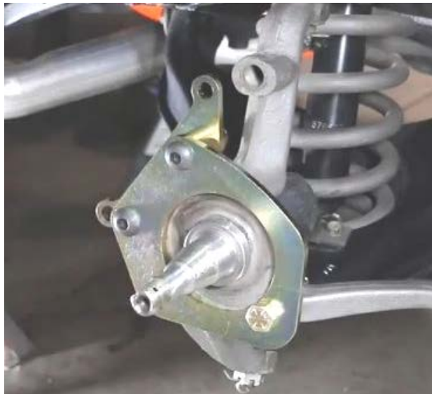
Figure 2 – Primary Caliper Mounting Bracket
