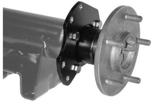
Mount the primary bracket to the flange. The calipers will mount to the rear.
