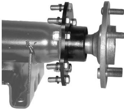
Install the bolts that will hold the secondary caliper bracket. Place lockwashers between the primary and secondary bracket.
