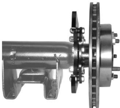
Mount the rotor onto the studs.
