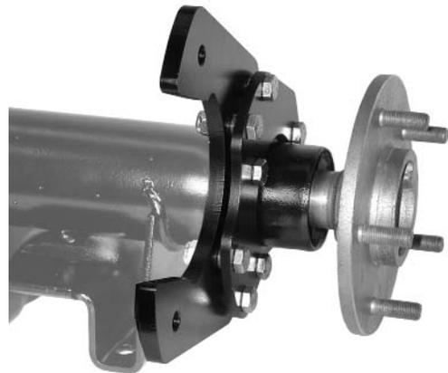
Mount the secondary bracket that will hold the caliper to the primary bracket.
