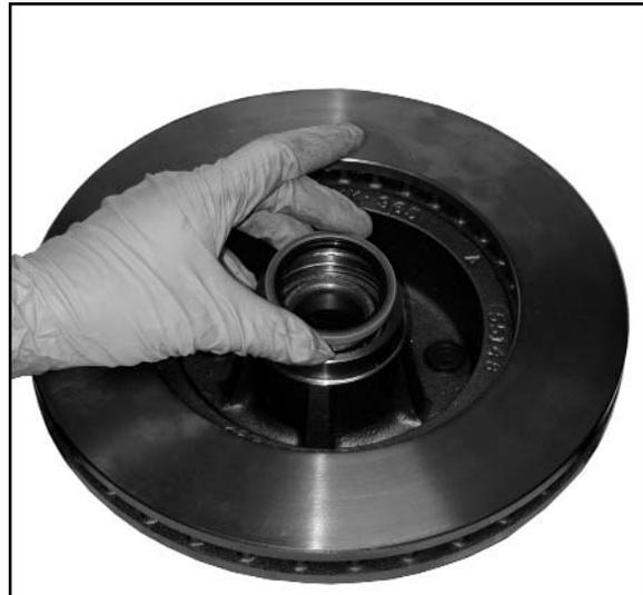
Install the bearing seal (HW7934).
