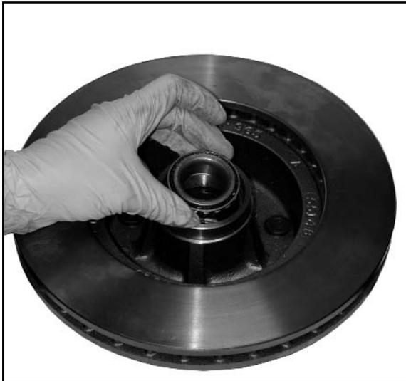
Install the inner A6 bearing.
