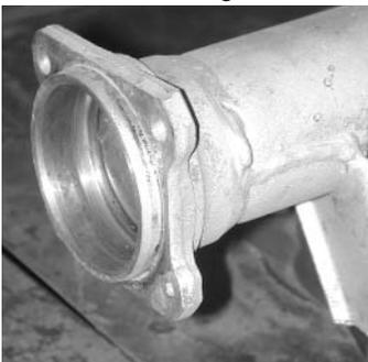
Remove stock drums, brakes, backing plates & clean!
