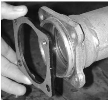
Install spacer plate to replace the backing plate.
