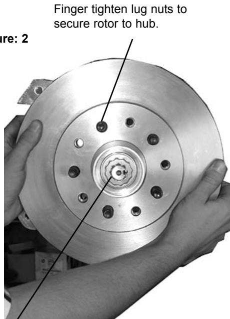
Bearing washer, wheel nut, cage, and cotter pin have already been installed.
