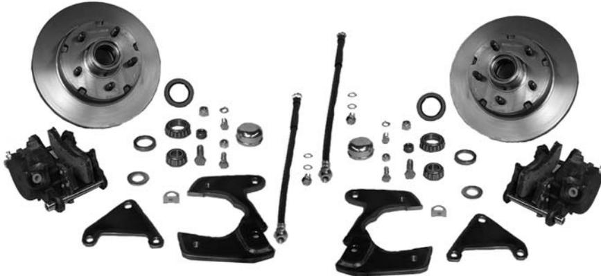
**BEFORE GETTING STARTED STRIP ALL THE OLD BRAKES, BACKING PLATES, STEERING ARMS, AND GUNK FROM FORD SPINDLES.**
