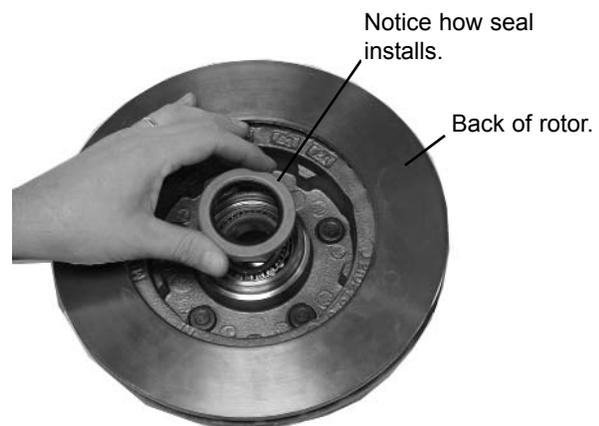
**BE SURE TO GREASE BEARINGS WITH A HIGH QUALITY BEARING GREASE.**
