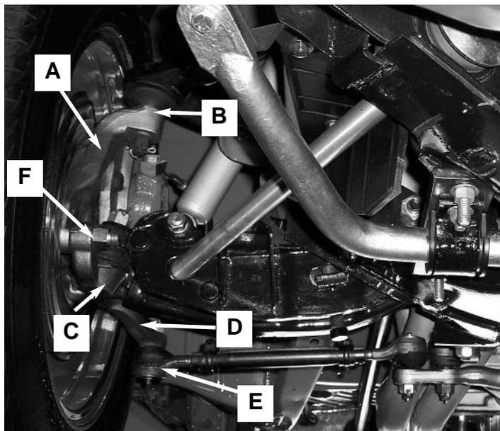
Disconnect the drum brake hose at the frame. Remove the outer tie rod end at the steering arm. Remove the lower ball joint from the lower control arm. Now you can complete the removal of the spindle by disconnecting the spindle from the upper ball joint at the upper control arm. At this point the spindle is loose and can be removed from the car.
