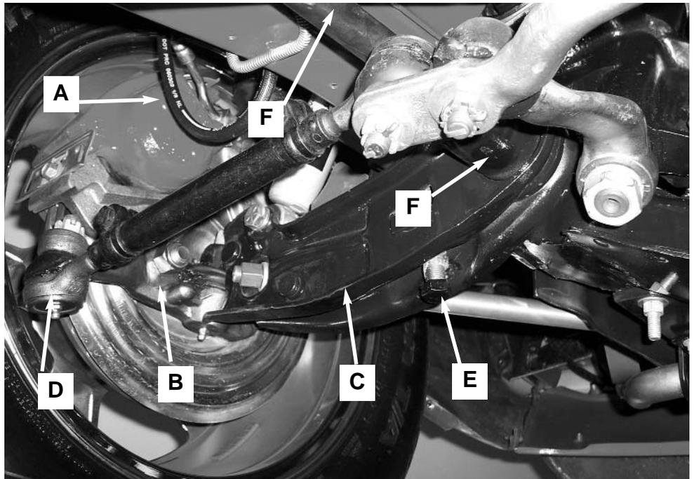
2. Raise the front of the car off the ground and support the full weight with jack stands under the frame so the front wheels are allowed to hang down with all the weight off them. Remove the wheels.
