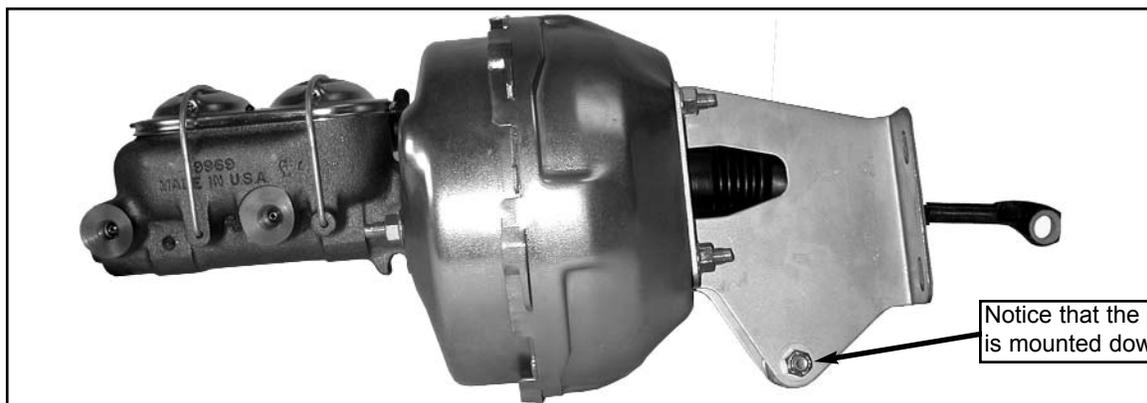
**Another way to correct the push rod angle on some models is to install the bracket with the pivot down!**
