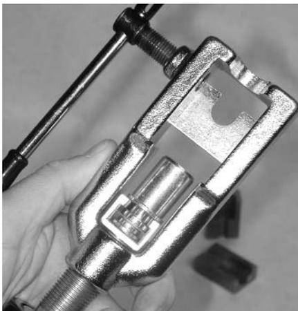
2. Insert the tube between the dies. (Select the right size die.)
