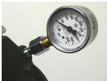
BE CAREFUL NOT TO OVERTIGHTEN the fitting into the caliper. This could damage the caliper or the fitting's threads. You want it tight enough not to leak brake fluid when the pedal is applied.
