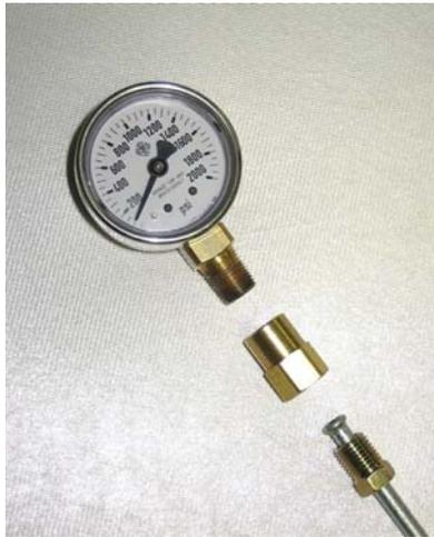
The female NPT portion of the adaptor mates to the pressure gauge, and the female inverted flare portion mates to the brake adaptor line. Once again, trial-fit all fittings by hand before tightening.
