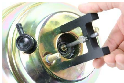
Figure 2a – Tool Positioned on the Booster
